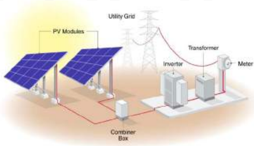
Figure 2-8 Illustration of the configuration of utility-scale PV power plants
