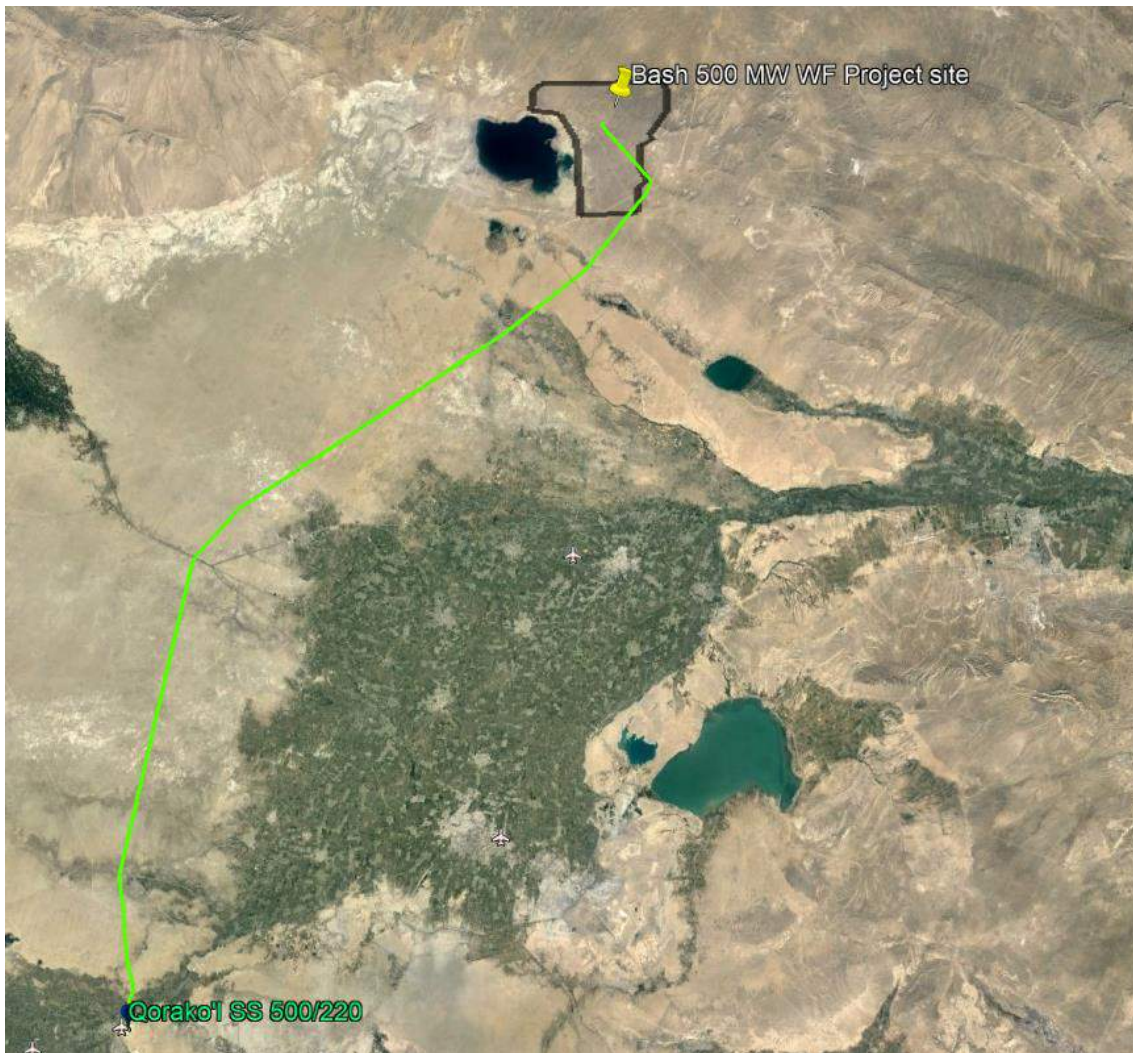
Figure 2-2 Alignment of 162 km OHTL from the Bash Wind Farm to Karakul Substation
