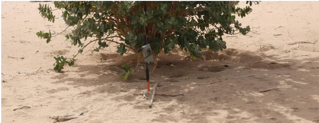
Figure 4-20: Sample Set-Up of Anabat Call Recorder at Sand Sheets and Dunes with Shrub Cover
